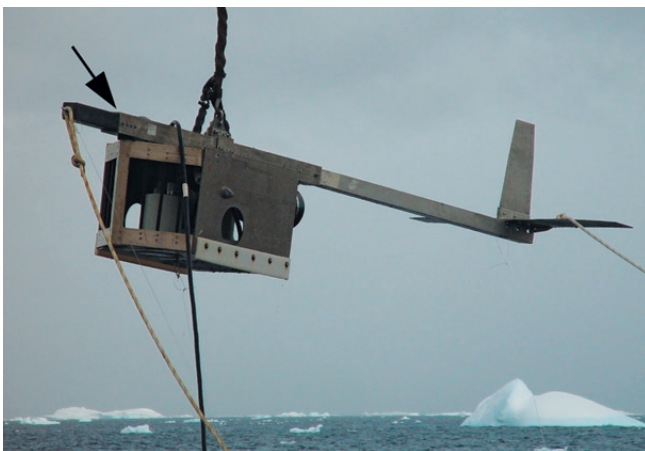
Fig. 1. The towed “Fish” ready for deployment. The arrow indicates where the camcorder was mounted.
