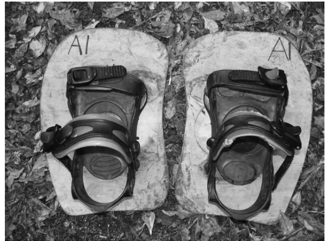
**Fig. 4.** Alternative to the conventional rectangular petrel boards. This kidney shape improved mobility without affecting weight dispersal properties. *Photo: E. Kennedy*
