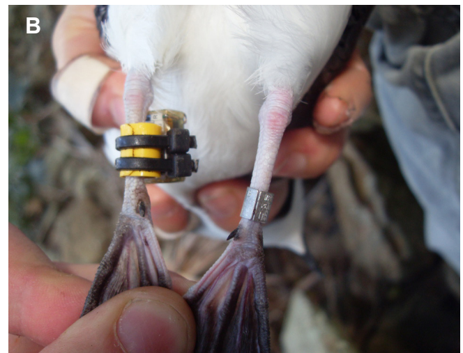
Fig. 2. Attachment of two types of geolocators: (a) MK14 with a Darvic ring and single cable tie; (b) LAT2900 with a Darvic ring and two cable ties.
