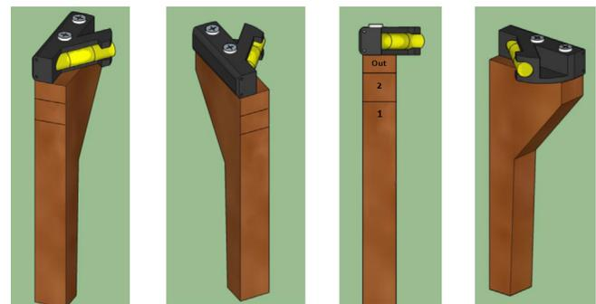
**Fig. 1.** The design of this study's handheld rangefinder, here with range lines for a bifurcated strip-width survey scenario. The black piece on top of the wooden handle is the 3D printed crown.
