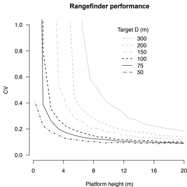
**Fig. 6.** Expected CV of estimations of strip width using the *Bangarang* rangefinder, when all error is introduced to all parameters simultaneously.
