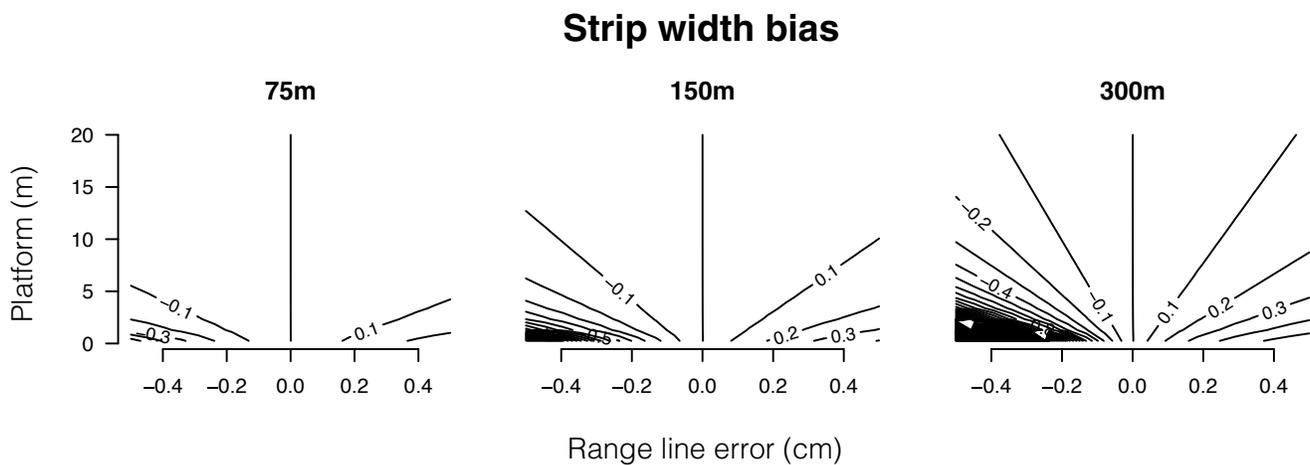
Fig. 8. Bias (contour lines, as a proportion of the target strip width) that would be introduced by error in range line measurements at three common strip widths.
