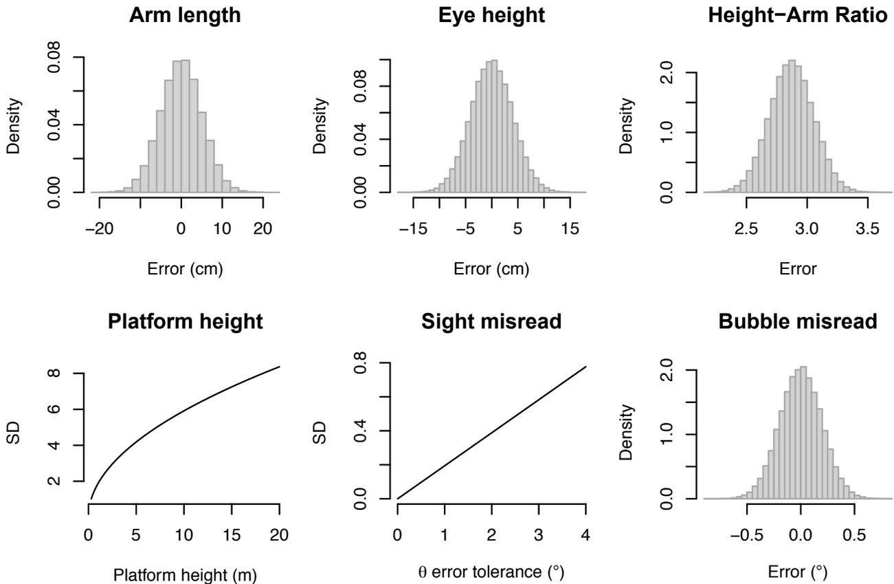
**Fig. 4.** Simulated distributions of random error for each variable, defined by the parameter values in Table 1, used in the sensitivity analysis. Standard deviation of platform height (bottom left) is expected to scale with platform height. Error tolerance in design of the sight hole (bottom middle) determines its expected contribution to the standard deviation of angle offset.
