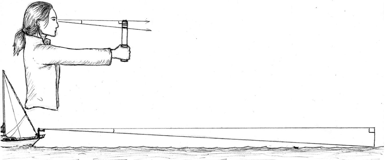
**Fig. 3.** The triangles involved in the design of the *Bangarang* rangefinder.
