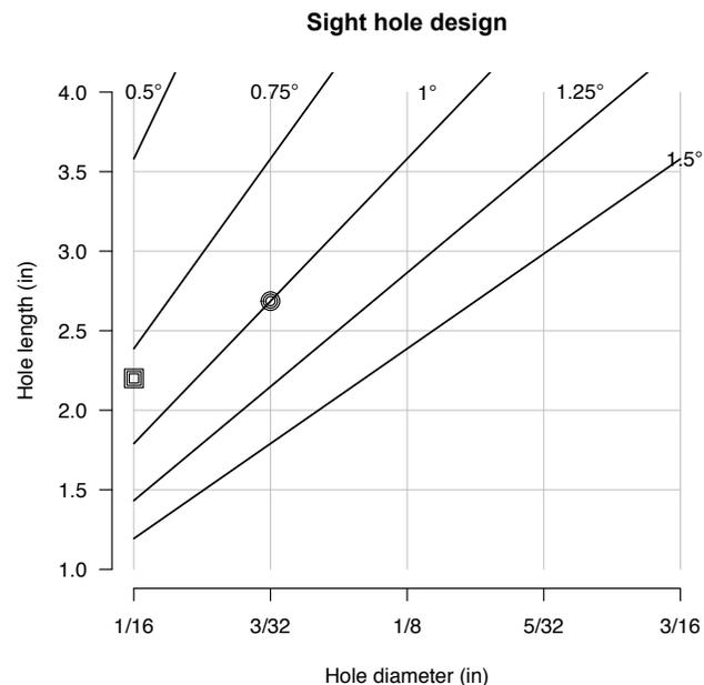
**Fig. 5.** Sight hole design at various tolerance levels of angle offset due to sight misread. Sight misread can occur because the rangefinder can be held at a slightly imperfect angle while light is still visible at the end of the sight. See text for details. Square mark denotes the design configuration trialed for this paper; circular mark denotes the revised design as a result of those field trials.
