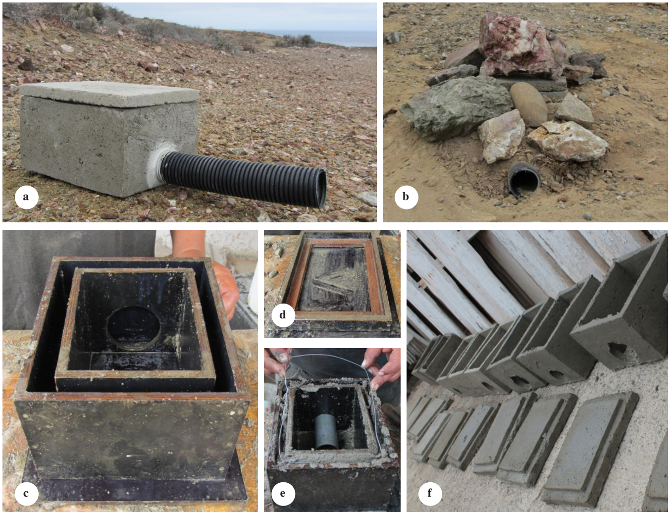
Fig. 1. Wood-concrete nest box built for Storm-Petrels. Nest box (a) finished and (b) installed in the field. Molds used to build the nest box: (c) internal and external pieces over one ground plate, (c) lid mold and (d) setting up of the metal wire and smooth PVC pipe. Finished boxes and lids (f) drying in the sun. Photos: Florian Schaefer and Yuliana Bedolla.
