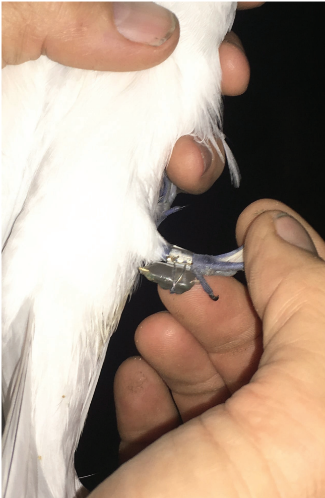
Fig. 2. White Tern Gygis alba showing stainless steel wire attachment of Global Location Sensor (GLS) unit to a bird band.
